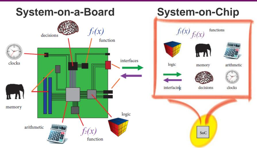
The SoC solution has <u>lower cost</u>, <u>faster and more secure data transfers</u> between the various system elements, <u>higher overall system speed</u>, <u>lower</u> power consumption, smaller physical size, and better reliability.
